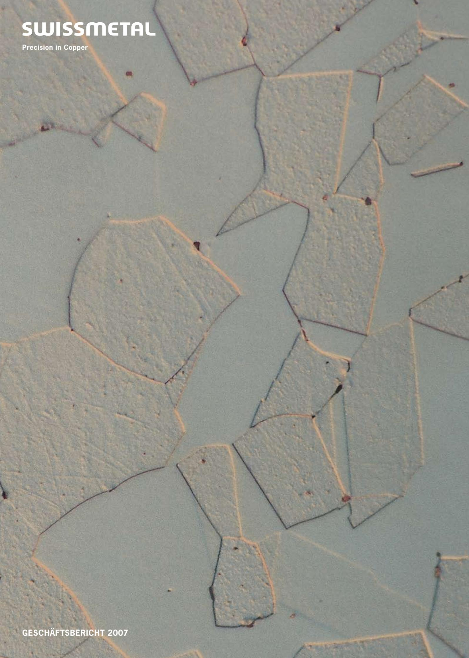
A microscopic view of copper metal grains, showing a complex, interconnected network of light-colored, irregularly shaped grains against a darker, blueish-grey background. The grain boundaries are clearly visible as thin, dark lines. The overall appearance is that of a polycrystalline material with a fine, textured structure.
